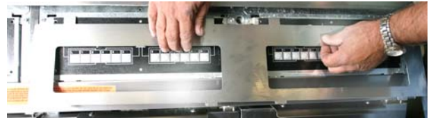
Figure 1: Remove the bezel over the right side computers by sliding it up to clear the bottom tabs and then down to clear the top tabs.
