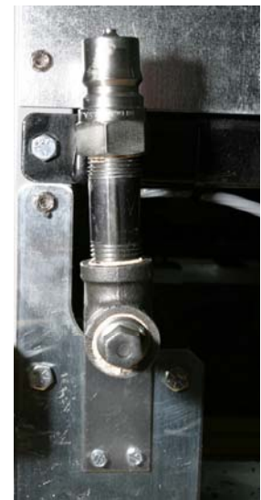
Figure 8: The rear discharge is secured at the back of the fryer with a bracket attached with drill point screws.
